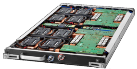
Front view showing thickness and Removal handle, hot, and cold water inputs
